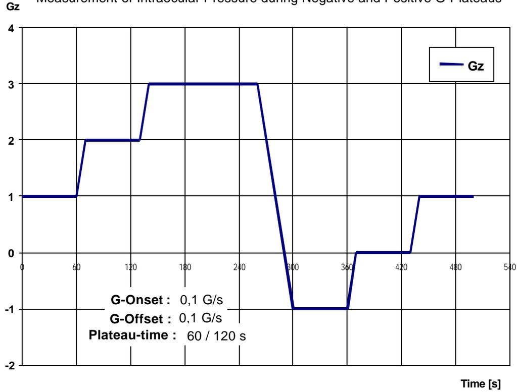
Self-Tonometry in the Human Centrifuge with different Positive and Negative G-loads
