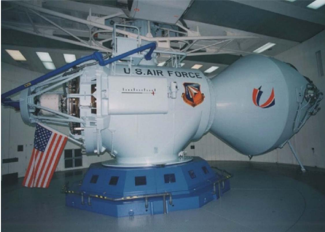
Figure 1. The Dynamic Environment Simulator centrifuge at AFRL, Wright-Patterson AFB, OH
